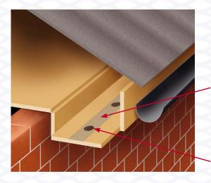
Soffit Vent Mesh is fixed over the ventilation holes to prevent birds and insects entering the roof void
